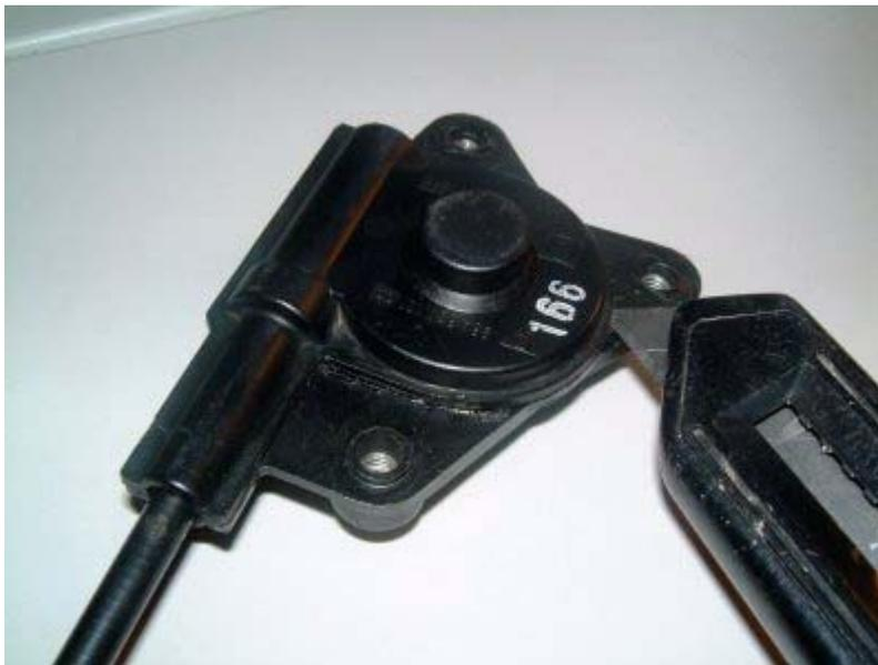
Carefully cut all around the periphery of the joint with a sharp knife to about 2mm deep. Take care not to go too far into the ridge of the joint. (See later photo).
