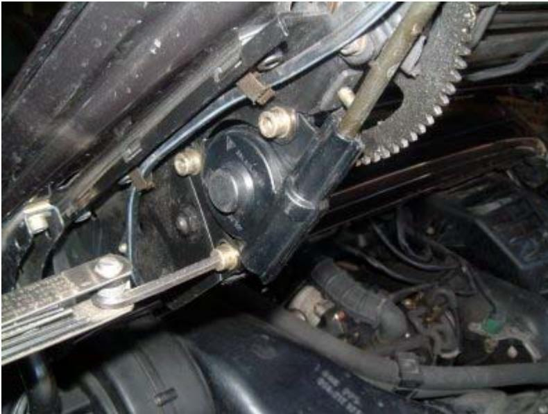
Undo the three M6 allen screws and remove the drive gearbox.
