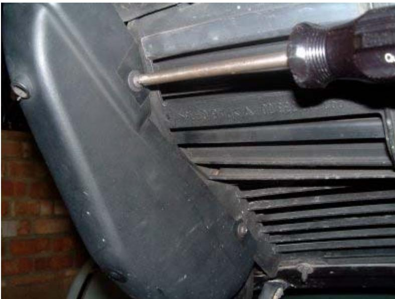
Undo the two posidrive screws and remove the cover.
