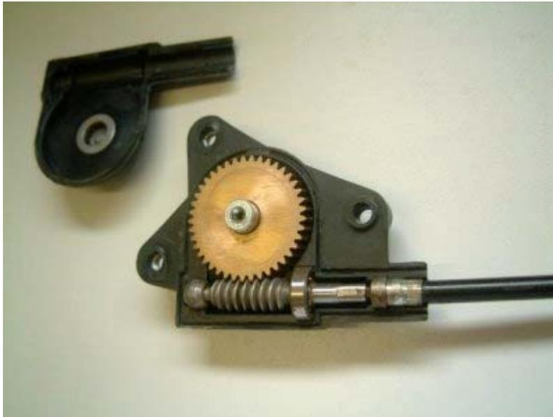
Remove the inner cable and clean and grease it. Reassemble as shown, with a generous dollop of grease around the worm shaft and worm wheel, making sure none gets on the casing joints. Also grease the exposed shaft on the worm wheel.
