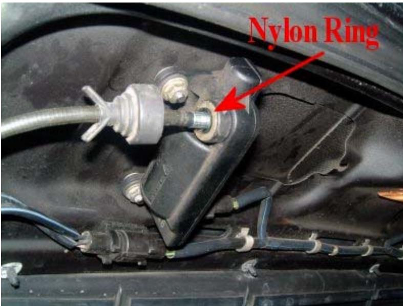
Pull back the rubber boot, prise out the white nylon ring with a small screwdriver, and remove the cable from the motor. The ring is split and comes out easily
