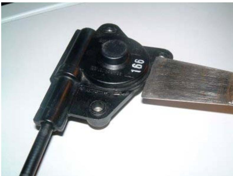
Carefully prise the joint apart using a knife edge scraper or similar. I gave a few light taps with a hammer and the joint separated fairly easily.
